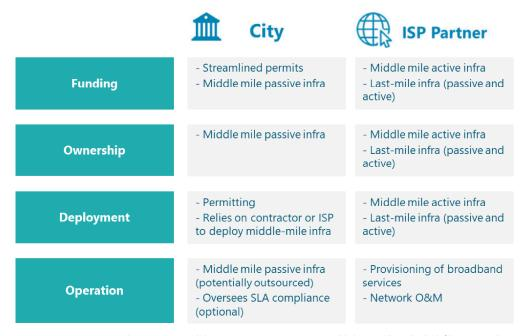
Figure 40. Conventional Operating Model: Leveraging City assets to establish a middle mile dark fiber network.
