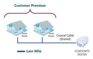
Figure 4. DOCSIS high-level architecture
