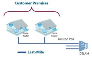
Figure 3. DSL high-level architecture
