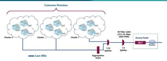
Figure 5. FTTH high-level architecture.
