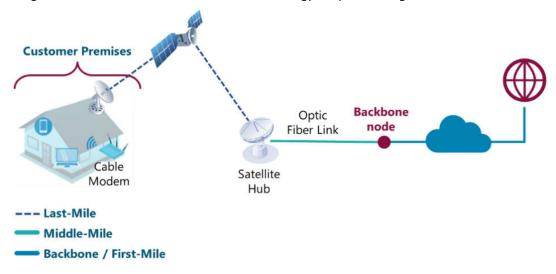
Figure 7. Satellite system high-level architecture
