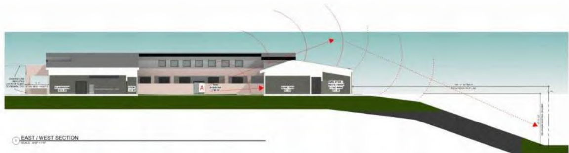
Figure 4. Section view illustrating shielding of dog noise from the new building
