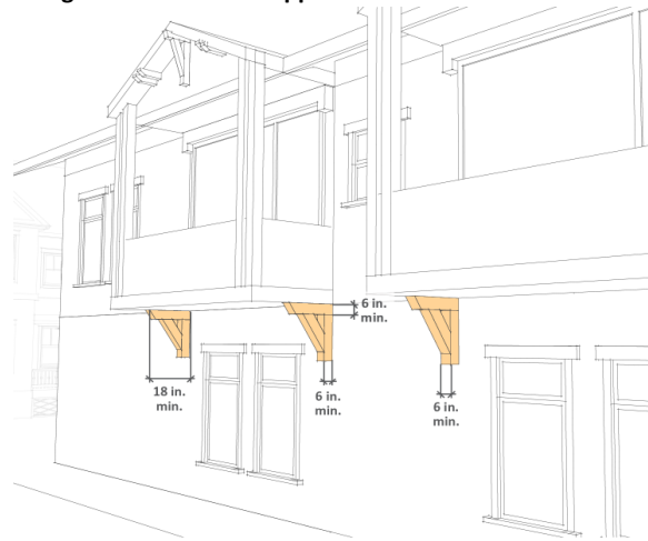
Figure 4-g: Post and Beam Supports
