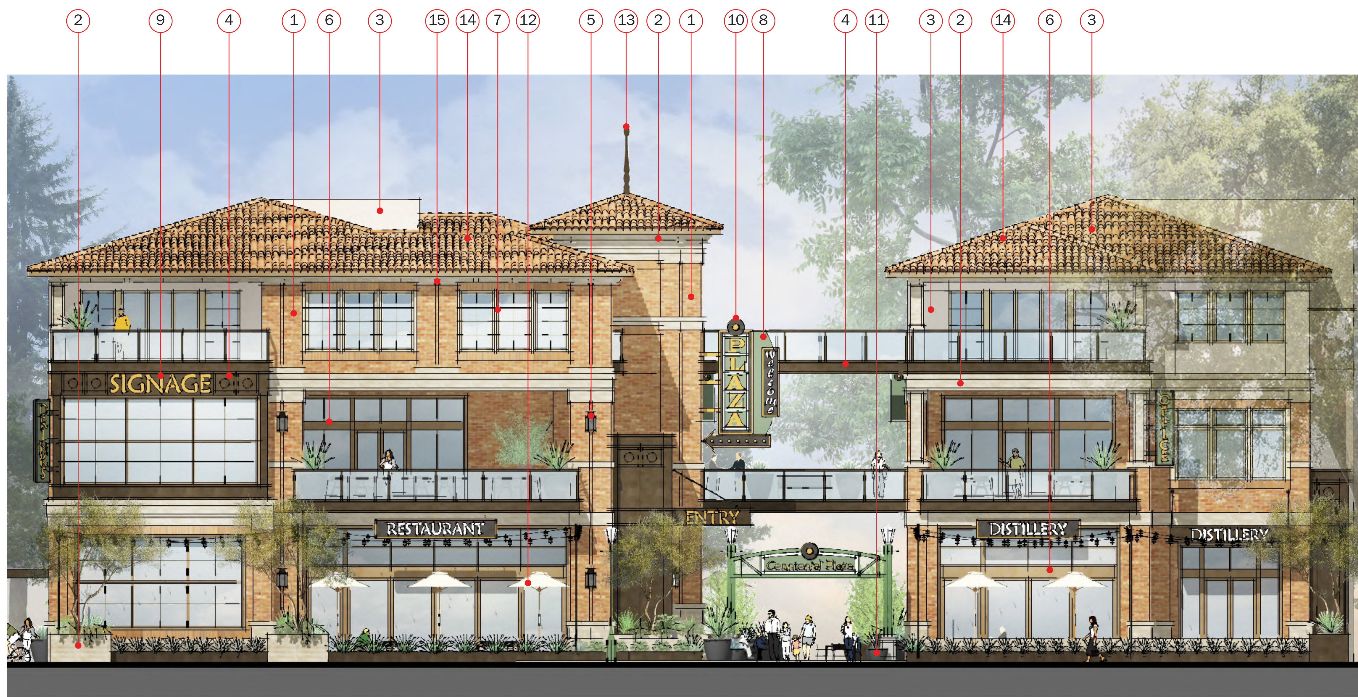
2 TRIM & BASE FINISH: PRECAST CONCRETE W/ LIMESTONE FINISH
