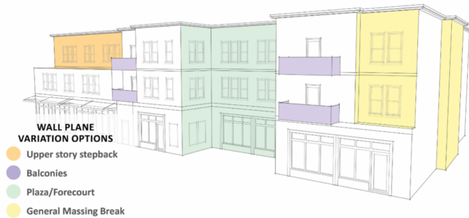
Figure 4-c: How to Measure Wall Plane Variation
