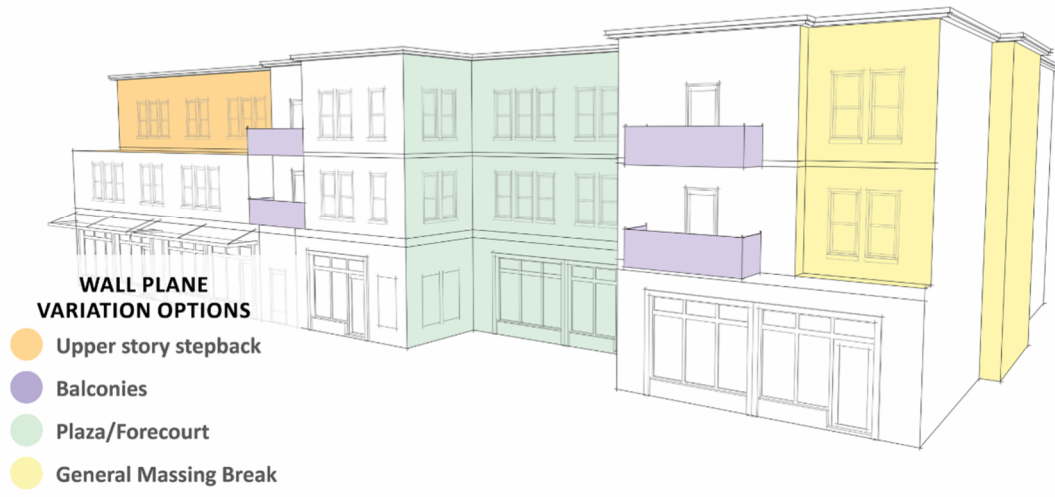
Figure 4-c: How to Measure Wall Plane Variation
