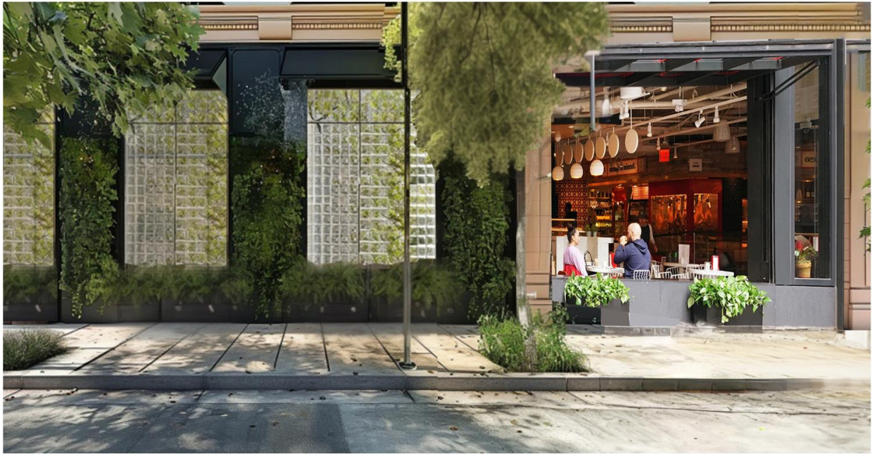
North Elevation (Traffic Way) Design Option "A" – Glass Block, Green Wall Art with Planters, and Bifold Storefront
