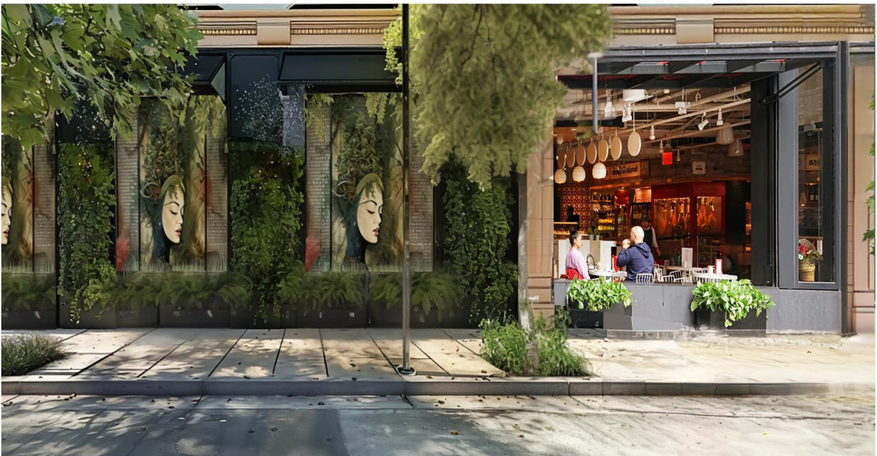
North Elevation (Traffic Way) Design Option "B" – Opaque Glass with Art Installation, Green Wall Art with Planters, and Bifold Storefront
